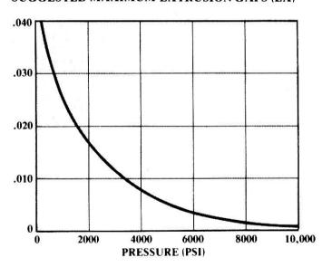
The EXTRUSION GAP CHART provides recommendations for the maximum acceptable extrusion gap at various pressure ranges. Eccentricity, ovality, bearing clearance, and normal wear of the mating parts must be considered when calculating the extrusion gap. This chart is intended as a guide and each application should be thoroughly tested.
